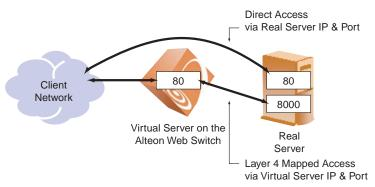
Figure 6-8 Mapped and Nonmapped Server Access
